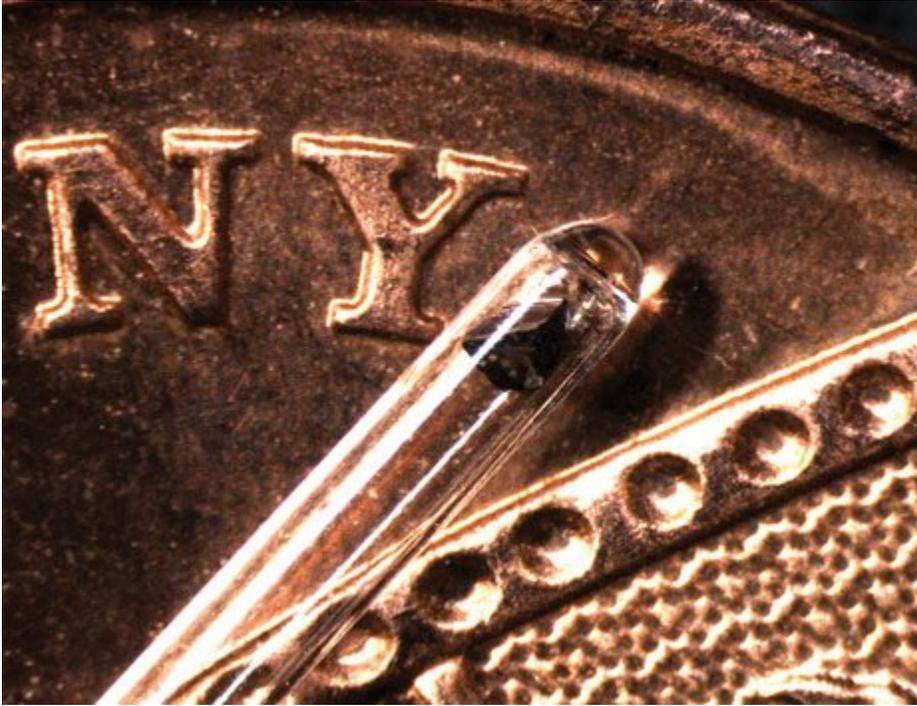
**BILLIONS OF BITS:** This tiny chip of silicon produced a record 10 billion pairs of quantum entanglements.
